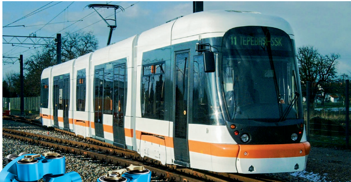
The connecting rod coupling LBK 330 and the membrane coupling MBG 200 have been successfully used with Cityrunner streetcars.
