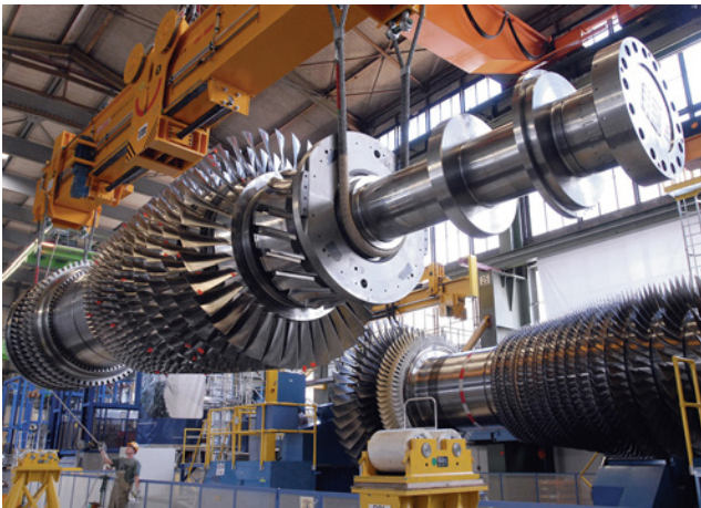
Gas and steam turbines
